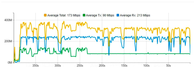
Fig. 7: Bandwidth test for the RF link with 80 MHz.
